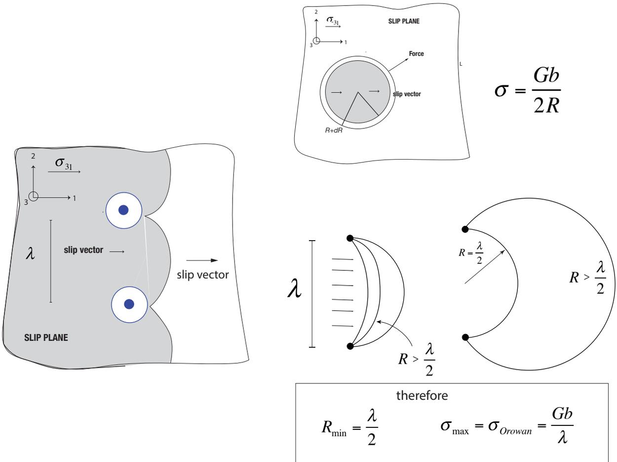
The Orowan stress can be applied generally to relate the yield stress to the effective distance between the obstacles to dislocation motion.
