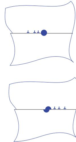
If the particle is difficult to shear like a ceramic or a hard metal, then it can completely pin the dislocation
